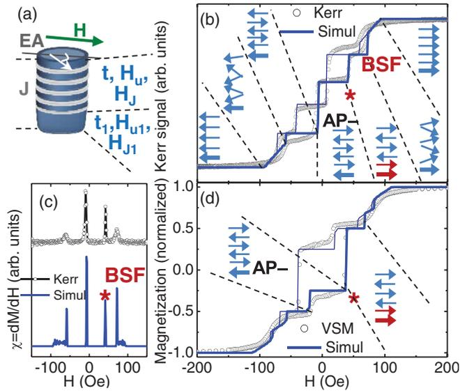
FIG. 1. (Color online) (a) Sketch of the investigated  $(\text{CoFeB/Ru})_6$  SL. (b) Kerr and (d) VSM signal as a function of the applied magnetic field for a SL with  $t_1 = 15$  nm and  $H_{u1} = 36$  Oe. (c) Magnetic susceptibility for the negative-to-positive field branch, from Kerr data and simulations.
