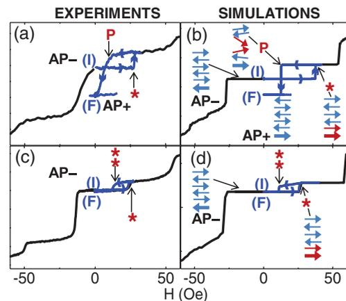
FIG. 2. (Color online) (a) and (c) Experimental Kerr data, (b) and (d) simulated Kerr for  $N = 6$ . (a) and (b) For  $t_1 = 15$  nm,  $H_{u1} = 36$  Oe, a soliton is nucleated and propagated. (c) and (d) For  $t_1 = 10$  nm,  $H_{u1} = 15$  Oe the bottom layer switches back, returning to AP- at remanence.
