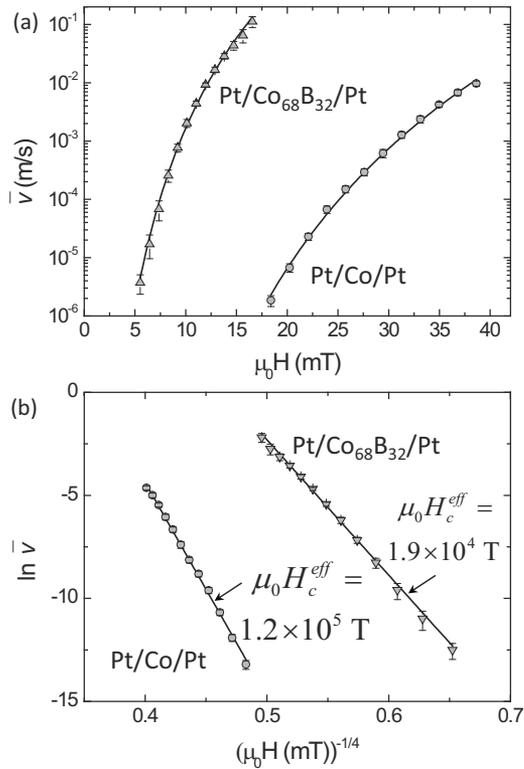
FIG. 2. (a) Average DW velocity vs applied field for patterned 900 nm wide strips of Pt(4 nm)/FM(0.6 nm)/Pt(2 nm) with FM=Co or Co<sub>68</sub>B<sub>32</sub>. (b)  $\ln v$  vs  $(\mu_0 H)^{-1/4}$  for the same data as presented in (a). The solid lines are a fit to Eq. (1) with the corresponding values of  $\mu_0 H_c^{\text{eff}}$  shown in (b).
