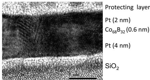
FIG. 3. TEM image of a  $\text{SiO}_2/\text{Pt}(4 \text{ nm})/\text{Co}_{68}\text{B}_{32}(0.6 \text{ nm})/\text{Pt}(2 \text{ nm})$  film. In the image a clear polycrystalline textured film is observed.
