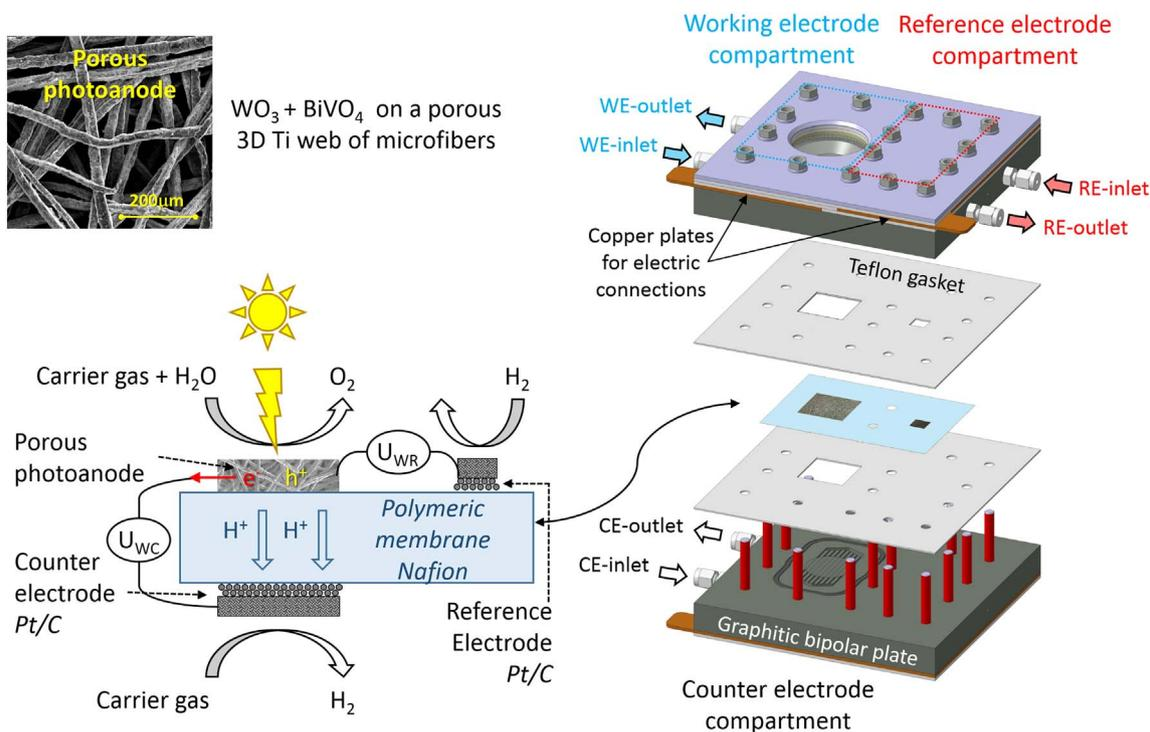
Fig. 1. (Left) Configuration and operation of the membrane (photo)electrode assembly. (Right) Novel PEM-PEC reactor design with three compartments for accommodating photoanode, cathode and reference electrodes [3].
